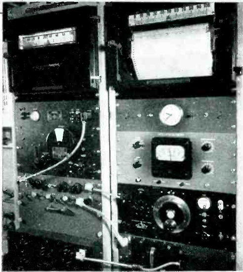
Above illustration shows special radio frequency oscillators and recording equipment used for determining temperature characteristics of Erie Ceramicons over a range from -40^{\circ}\text{C} to +100^{\circ}\text{C} .
